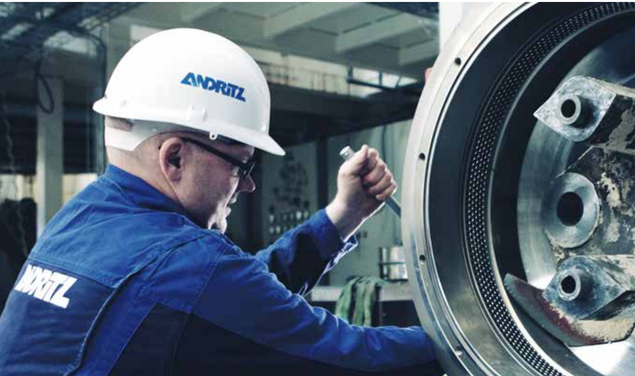
Pellet mill maintenance
