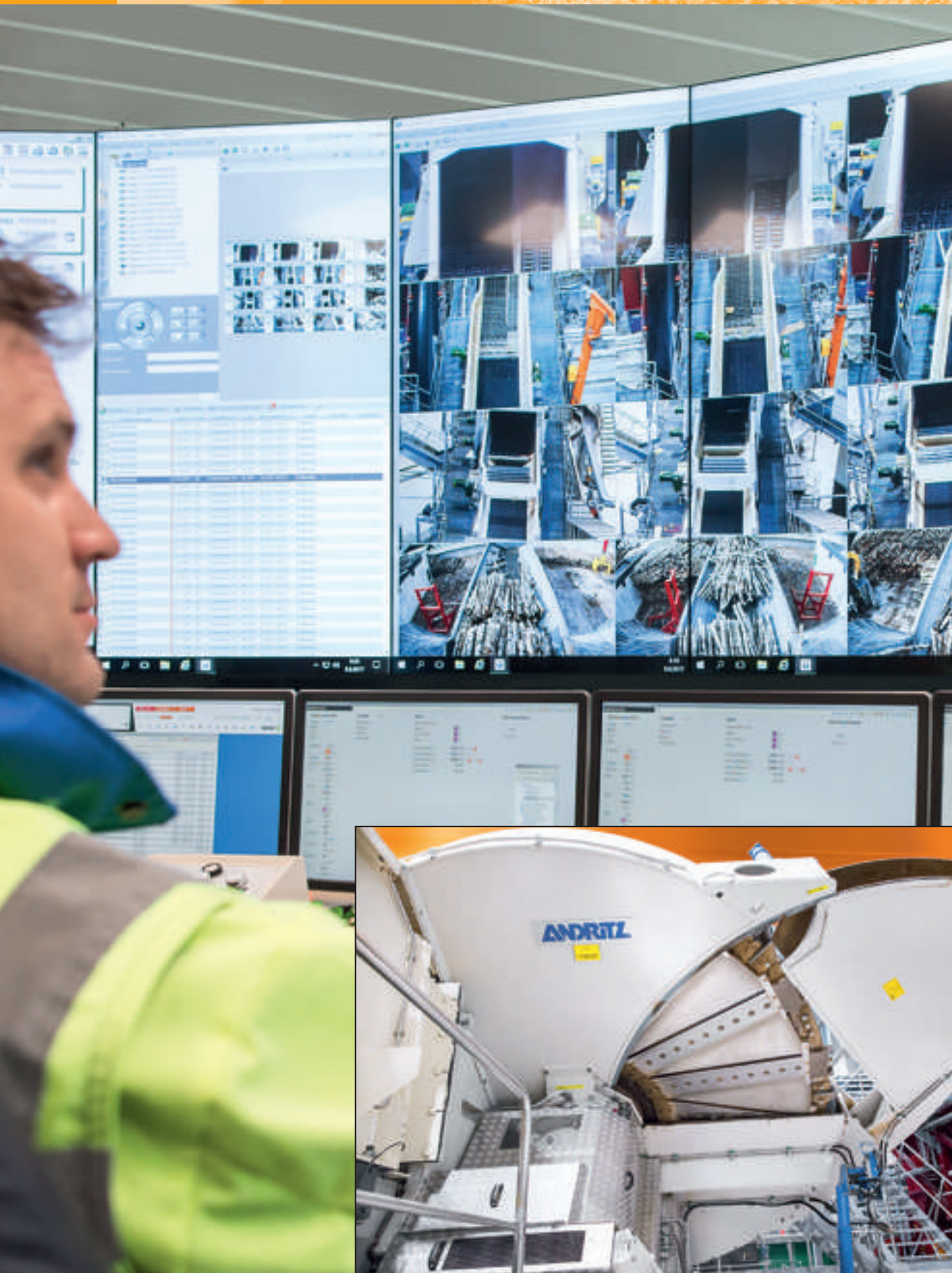
State-of-the-art online monitoring of the woodyard with ANDRITZ IIoT solutions. The entire production process is monitored and controlled from a central control room. The world's biggest chippers (photo), each with a diameter of 3.87 meters, and the three debarking and chipping lines with the largest capacity worldwide are also monitored online by video cameras.
